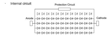
(Note) Protection circuit has resistor typical  $20M\Omega$
